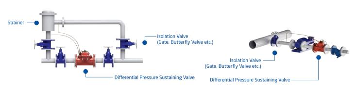
Armaș Differential Pressure Sustaining Valves sustain pressure difference of two different points which is located in the system.
