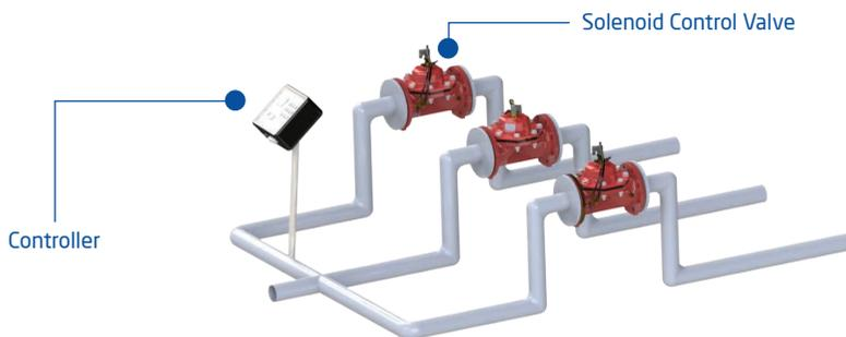
Armaş Solenoid Controlled Valves can be used with a local control unit or advanced automatin systems.
