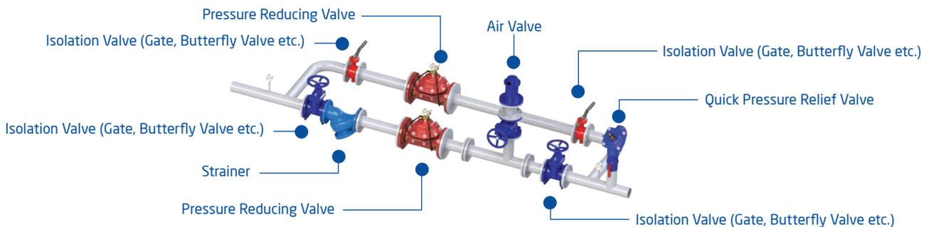
Armaş Pressure Reducing Valves reduce pressure to setted downstream pressure value without affecting upstream pressure value at pressure chambers and supplying lines.
