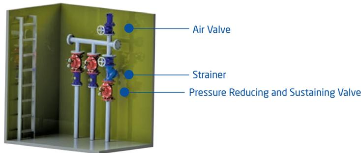
Armaş Pressure Reducing and Sustaining Valves can be used for avoiding any interaction of high altitude and low altitude usage areas which is fed by same line and for avoiding unnecessary line discharge.
