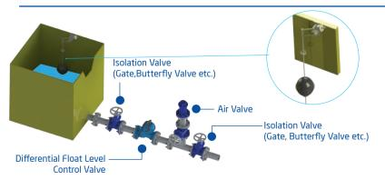
Armas Differential Float Level Control Valves control minimum and maximum water levels at water tanks thanks to its differential float.
