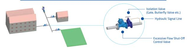
Armaş Excessive Flow Shut-off Valves prevent flood damages caused by pipe burst.
