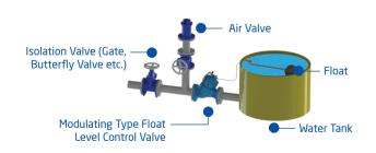
Armaş Float Level Control Valves prevent water tank overflow.
