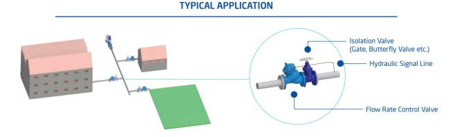
Armaș Flow Rate Control Valves limit the flow rate to requested value.
