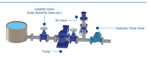
Armaş Hydraulic Check Valves prevent back-flow.
