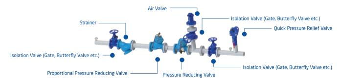
Armas Proportional Pressure Reducing Valves reduce pressure without any pilot as proportional according to catalogue values.
