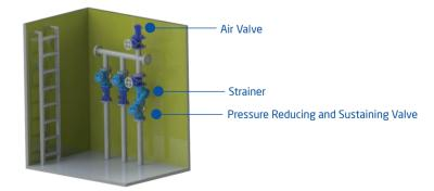
Armas Pressure Reducing and Sustaining Valves can be used for avoiding any interaction of high altitude and low altitude usage areas which is feeded by same line and for avoiding unnecessary line discharge.
