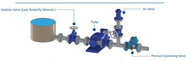
Armaș Pressure Sustaining Valves control upstream pressure to provide a good condition operating for pump systems.
