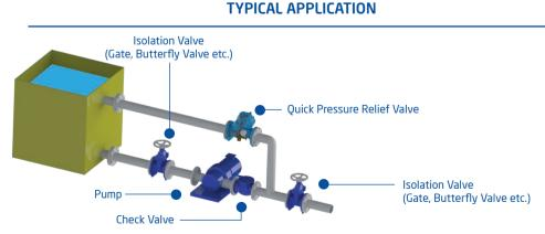
Armaș Quick Pressure Relief Valves protect pipe-line and system equipments during pressure fluctuations.
