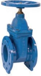
Valve is closed or opened by moving wedge upward or downward via threaded stem mounted in the body. Wedge is rubber coated and It is not used as a check valve and flow rate adjustments.
