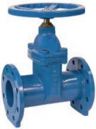
Valve is closed or opened by moving wedge upward or downward via threaded stem mounted in the body. Wedge is rubber coated and It is not used as a check valve and flow rate adjustments.
