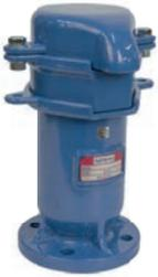
Armaş AAV Series Automatic Air Release Valves are the valves that operate with line pressure. Armaş AAV Series Automatic Air Release Valves are the air valves that provide the venting of the air during filling and preventing of vacuum by taking air into the installation during emptying, releasing of the air that accumulates in the installation during active operation with the help of pressure and that operates in automatic manner.
